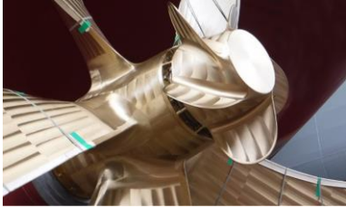
Energy-saving device attached to the propeller (PBCF)
