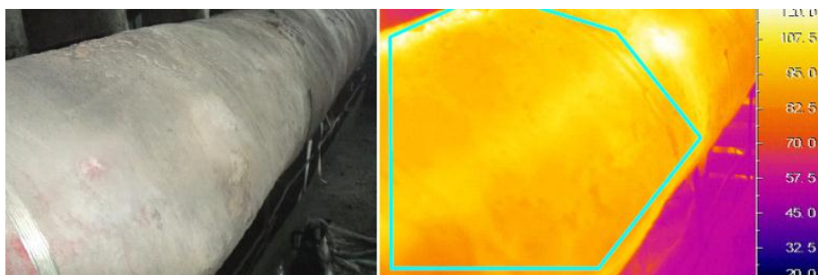
Figure AP2-5.1. Example of thermographic image pixels extracted for the total area within the main steam pipe without installation of project thermal insulation material
