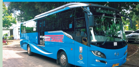
CNG-Diesel Hybrid Public Bus (Indonesia) Hokusan Co., Ltd.
