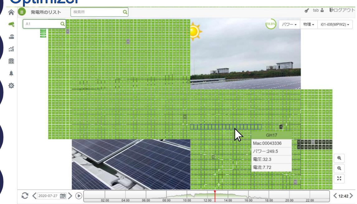
Example of showing bad panel. Engineer can estimate error cause in advance, so that it can minimize repairing team build as well as repairing time.
