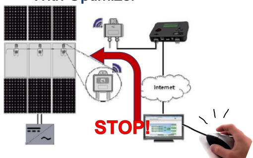
Even turning off the inverter, solar panel keeps generating power as long as there is sun light.
