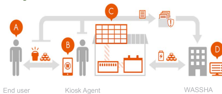
System for device charging service using photovoltaic panels at kiosks
