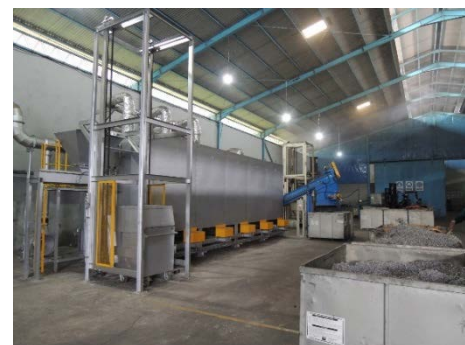
300 kg/h continuous aluminum chip degreasing furnace
