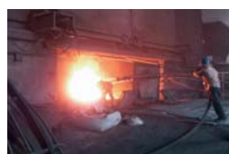
Biomass use in the electric arc furnace for steel manufacture (Indonesia)
