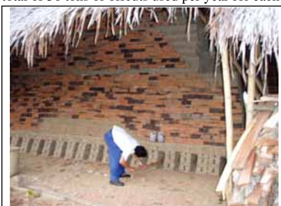
Fig-12: Being prepared for brick firing (Jun 22,2006)
