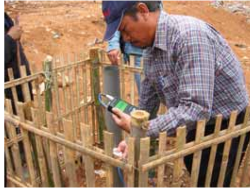
Fig.6 Measuring the flow speed of LFG
