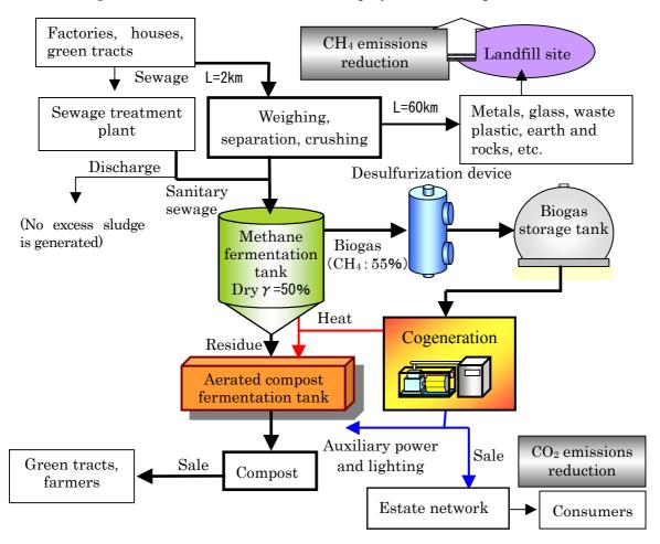
biomass at the Amata Nakorn Industrial Estates in Chon Buri Province, with a view to using it as raw materials for conducting methane fermentation in order to treat waste and produce biogas, and to use the collected biogas as fuel for generating power and recovering thermal energy.
