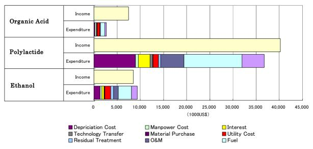
Fig.3 Balance of the each biomass industry
