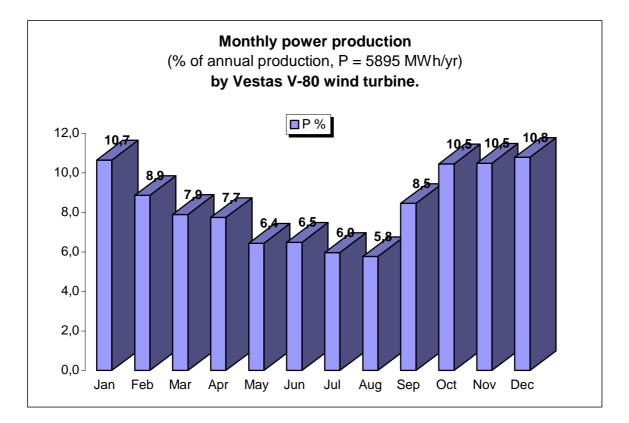
Figure 1. Monthly power production (% of annual production, P = 5895 MWh/yr) by Vestas V-80 2 MW wind turbine.
