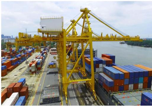
• Ship to Shore (STS) Crane is used to lift the container between the vessel and the shore must be a reliable device due to the use of over 95% of the service life. The STS-100% electric type is used to reduce CO<sub>2</sub> emissions.
