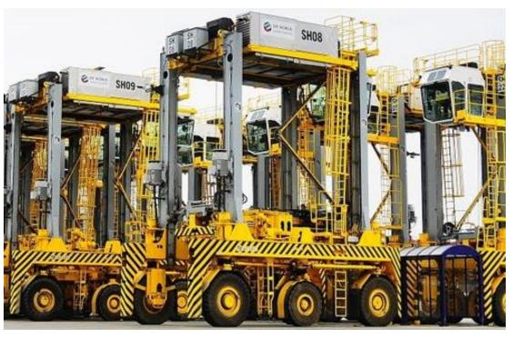
• Shuttle Carrier are used for horizontal transportation between the wharf and the container yard. The carriers must be equipment that is agile and has continuous work to support the STS crane to work continuously and efficiently.
