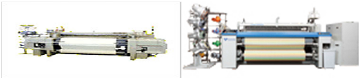
Reference loom: rapier loom OptiMax (left) Project loom: air jet loom JAT810 (right)
