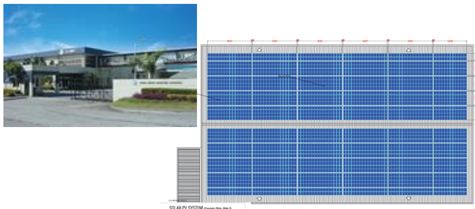
Solar Panel Layout for Enomoto Factory (175W x 5,408 panel = 946.4kW)
