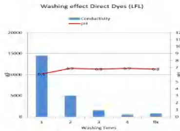
Figure 4-11 Washing effect by Direct Dyes
