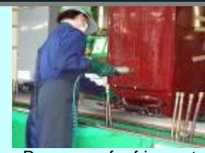
Recovery of refrigerant fluorocarbon from fridge
