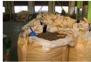
RDF stored in flexible container
