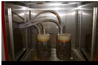
An experiment on gas generation (450g of RDF is in 1L bottles )
