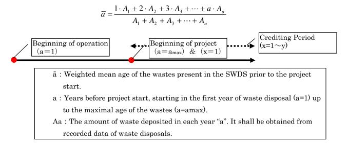
• Exponential function term " $\exp[-k_j.(y-x+\bar{a})]$ " could be applied instead of " $\exp[-k_j.(y-x)]$ " in the FOD model, where x will begin from the project implementation.
