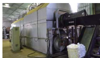
No.17-13 Continuous compaction and carbonization system for low density waste
