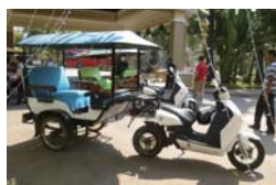
No. 14-2: Electric motorcycle with a passenger carriage (prototype)
