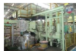
No.7: Energy Saving through Introduction of Regenerative Burners to the Aluminium Holding Furnace of the Automotive Components Manufacturer (Indonesia)
